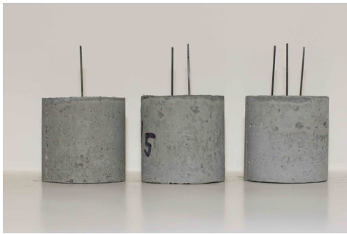
Fig. 11 Setup of fibers in the sample with the distance between adjacent fibers of 10 mm.
