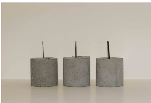
Fig. 9 Setup of fibers in the sample with the distance between adjacent fibers of 0 mm.
