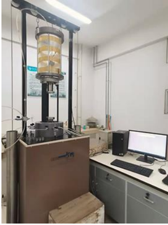
Fig. 2 Hollow cylinder torsional shear apparatus.
