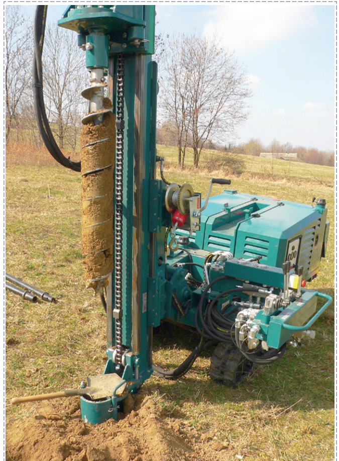
HVS 125 drilling and taking samples from a fault zone in Bílá Voda, Czechia. Photo F. Hartvich.
