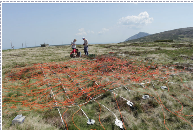
3D measuring of polygonal soils together with colleagues from the Charles University in Prague using an ERT system ARES at Modre Sedlo. In the background Mt. Sněžka (1602 m a.s.l.)
