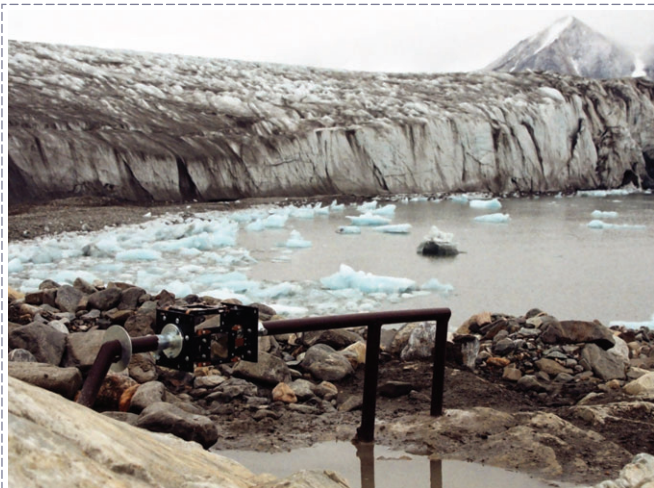
TM-71 crack gauge installed on fault in the forefront of the Hans Glacier in Hornsund, Svalbard. Photo F. Hartvich.
