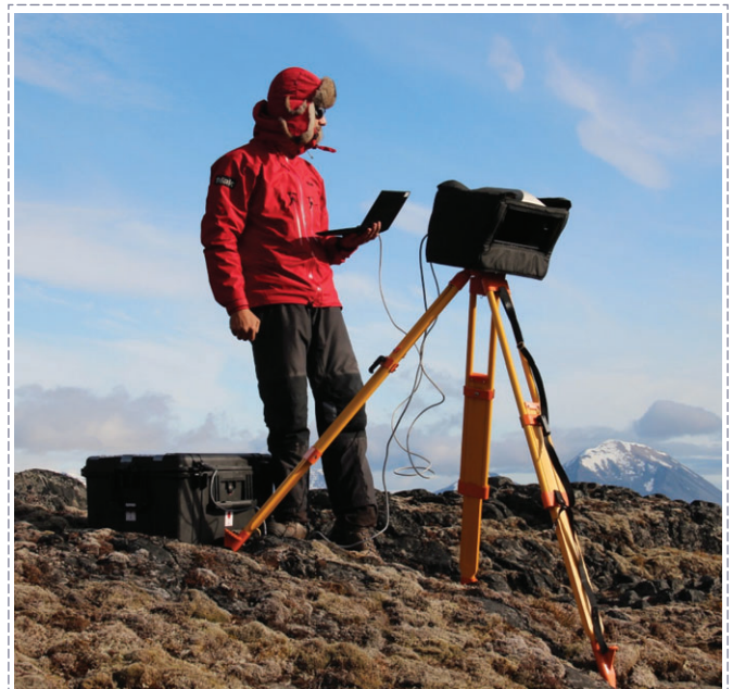
Jan Blahůt is surveying fault area in Hornsund, Svalbard with ILRIS3D terrestrial laser scanner. Photo M. Hladká.
