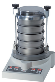
Autosieve system Fritsch (vibratory sieve shaker) used for grain size analysis of soil samples.
