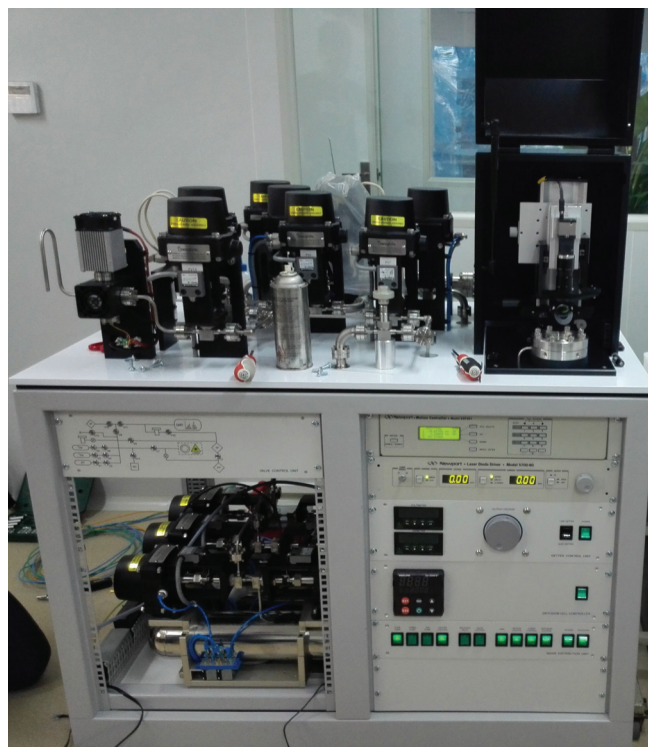
Alphachron™ automated helium thermochronology instrument is a turn-key system for the automated extraction and measurement of radiogenic helium from mineral samples.
