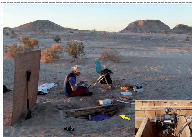
Displacement monitoring on the Superstition Hills Fault, California, by mechanical dilatometer TM71 with automated data recording. Photo P. Štěpančíková
