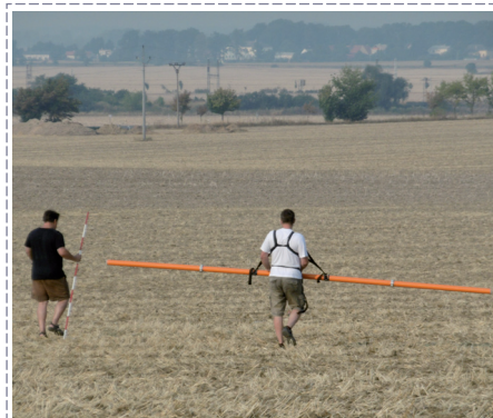
Measurements of conductivity by CMD Explorer serve as a powerful tool for determination of areal extent of sedimentary features (e. g. alluvial fans, colluvial deposits etc.). Photo J. Šreinová
