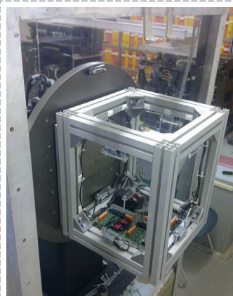
Testing of Rotaphone in USGS laboratory in Albuquerque, New Mexico, USA. Special rotary shock table facilitates a detailed determination of the Rotaphone parameters.
