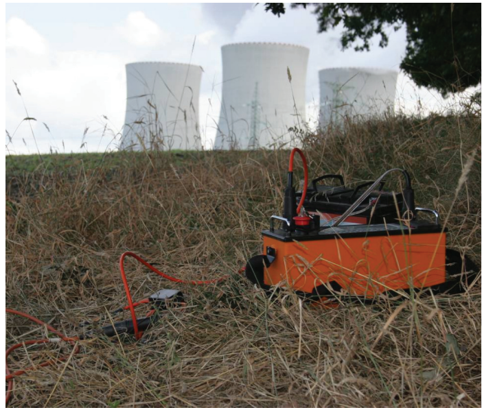
Acquiring geoelectrical data in the vicinity of the Temelín nuclear power plant
