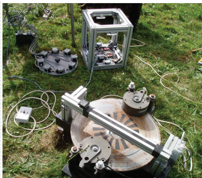
The Rotaphone: prototype of the seismic rotational sensor system and generator of rotational movements.
