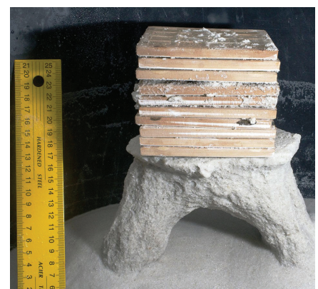
Result of experiments with Střeleč sandstone – a perfect experimental gate, formed by repeatedly flooding a loaded block with a rectangular opening
