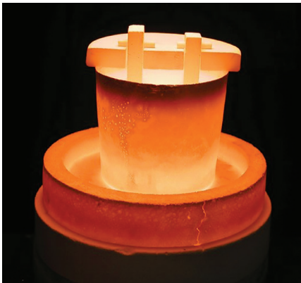
Static plate corrosion test – crucible with refractory material corroded by glass melt
