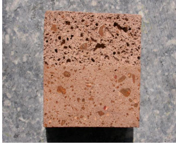
Figure: A solid product from a foamed and a compact geopolymer containing a high amount of aluminum-production waste
