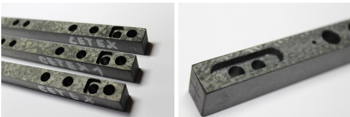
Figure 3. Novel carbon/PPS composite intraoperative guides for accurate targeting of the distal nail holes and accurate interlocking screws used for the treatment of diaphyseal fractures of long bones.
